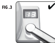
FIG. 3 Light tip held flat and fitting exactly on the light sensor. Unit will display correct results
