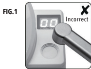
FIG. 1 Light tip too far away. Unit will display low or no results.
