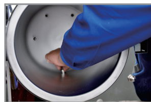
2. Back-out the water filter.
