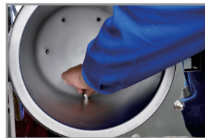
2. Back-out the water filter.
